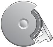
Step 2. Match blade cutting edge angle to wheel. Grind cutting angle.
