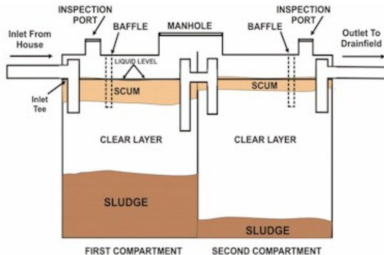
The upper portion, or scum layer, is where detergent waste, greases, and oils naturally accumulate in the tank. The lower portion is called the sludge layer. This layer is composed of the solids that settle at the bottom of the tank. Bacteria which are naturally present in sewage work to digest, or break down, the sludge and scum layers.
