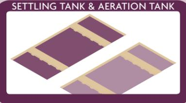
The **primary settling tank** provides for the removal of heavy solids that sink to the bottom, as well as floating materials such as oil and grease.
