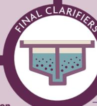
This secondary treatment allows microorganisms to fall to the bottom of the tank for recycling back to aeration or to be removed for use in the solids treatment process.
